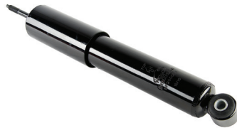
Ref. # BF280003 CHEVROLET D-MAX 4X4 / FORD BRONCO 34730 OEM 8-97368-598-0 POSITION: FRONT / GAS STYLE: 2 SIDE: R/L SIZE: 15,8"
