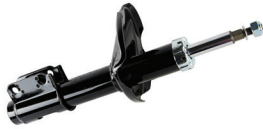
Ref. # BF590003 MAZDA 323 1,3 / 1,5. ALL YEARS OEM B.00134799C Monroe: 71888 POSITION: FRONT / HID STYLE: 5 SIDE: L
