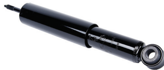
Ref. # BF290020 CHEVROLET NPR / NKR ELF 88 UP OEM 8-97083-027-0 Monroe: 66716 POSITION: FRONT / HD STYLE: 2 SIDE: R/L SIZE: 23"
