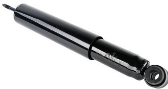
Ref. # BF290019 CHEVROLET NPR / NKR ELF 88 UP OEM 8-97083-035-0 POSITION: FRONT / HID STYLE: 2 SIDE: R/L SIZE: 23"
