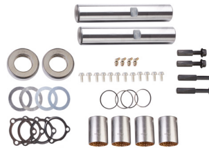
Ref. # BF548 Ford LNT 9000 Model 76-98 Meritor Shaft 10000, 11000, 12000 LBS
